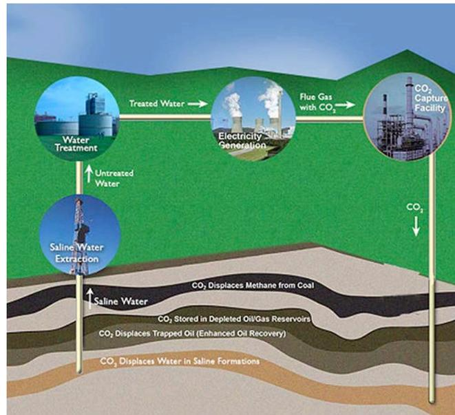
**Figure 6-15. Diagram of the process. Saline Water withdrawal and CO<sub>2</sub> sequestration (source: DOE/NETL)**
