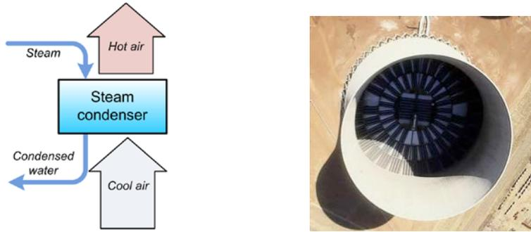
**Figure 2-10. Diagram of dry cooling and aerial view of a dry cooling system**
