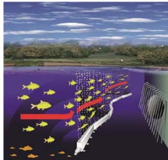
**Figure 7-6. Ovivo's Bio Acoustic Fish Fence system. It uses a combination of sensory stimuli that produces a linear barrier to guide fish away from the point of abstraction to an exit or by wash. The sensory stimulus is a combination of customized sound signals, directional strobe lighting and an air bubble curtain. (Source: Ovivo's website)<sup>9</sup>**
