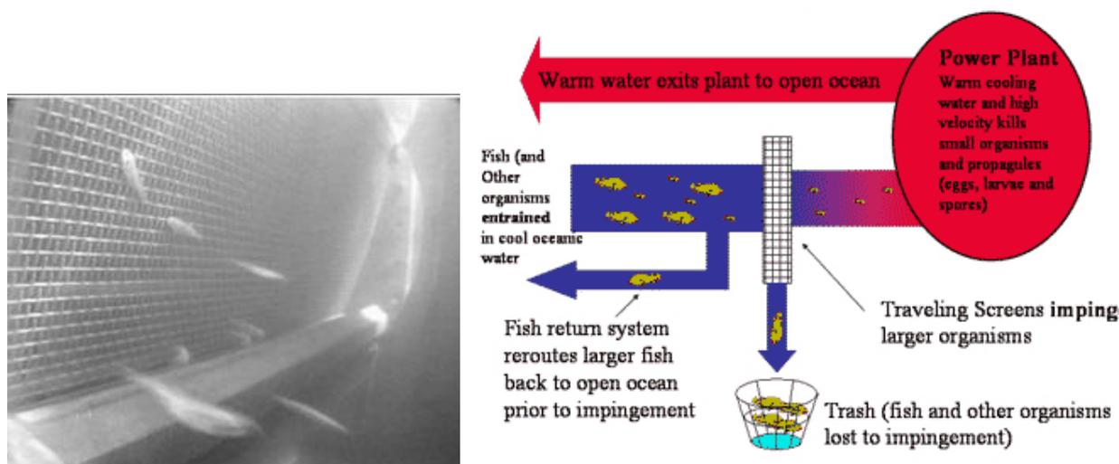
**Figure 7-4. a) Picture of fish impingement (left). b) Diagram showing impingement and entrainment (right).**
