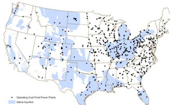
**Figure 6-14. Locations of Saline Aquifers and Coal-Fired Power Plants. Light blue are saline aquifers and black points are operating coal-fired power plants. (Source: ALL Consulting, LLC/NETL)**
