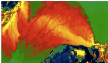
**Figure 7-3. Thermal Plume of the Indian Point Nuclear Power Plant in New York**
