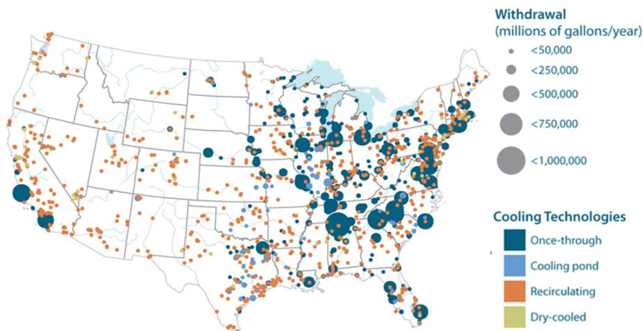
**Figure 2-11. Types of Cooling Systems and water withdrawal in the US. Source: EIA 2008, UCS 2011**
