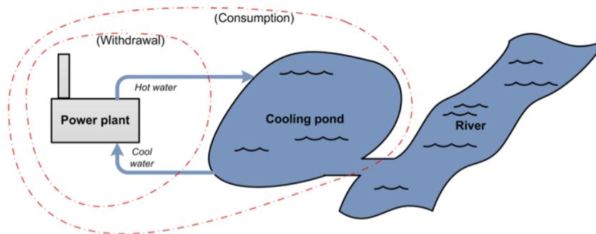
**Figure 2-9: Diagram of a cooling pond system**
