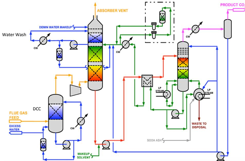
**Figure 4-14: Typical Econamine FG+ Carbon Capture Process. (Source: Fluor website<sup>4</sup>)**
