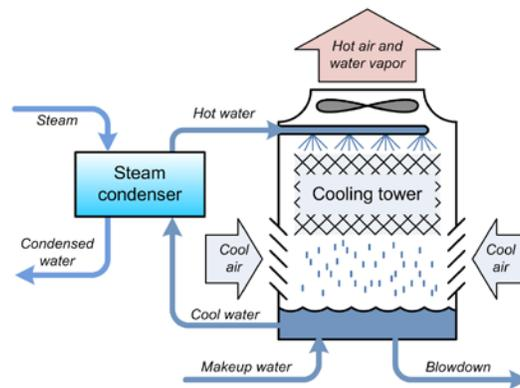
**Figure 2-7: Diagram of wet cooling tower (mechanical draft)**
