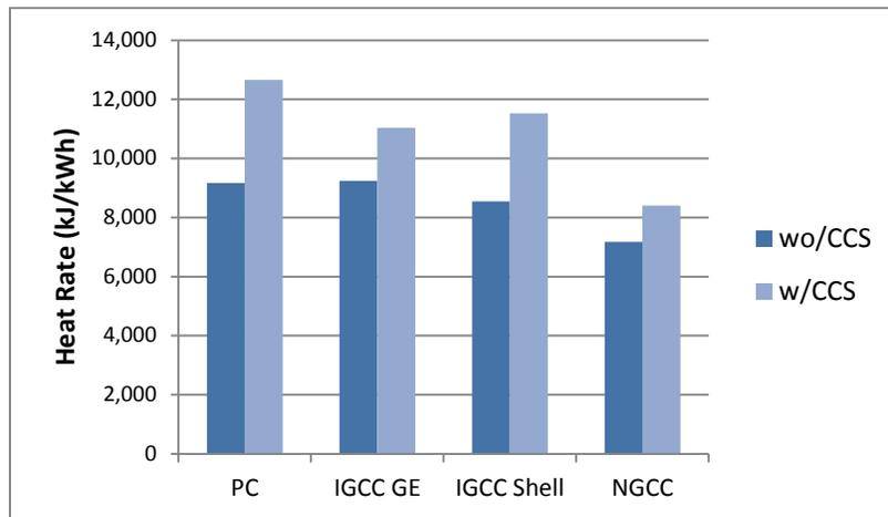
**Figure 4-12: Comparison of Heat Rates (HHV) with and without CC. (DOE/NETL, 2010)**
