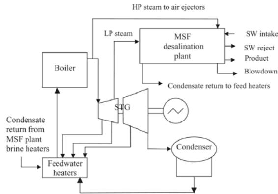
**Figure 6-8. Dual-purpose plant with extraction steam (source: Kamal, 2005).**
