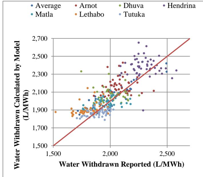
Figure 5-2. Comparison of water withdrawn from field data (horizontal axis) with model results (vertical axis) (monthly data from 2006 to 2010)
