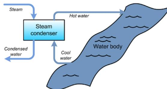
**Figure 2-6: Diagram of once-through cooling system**
