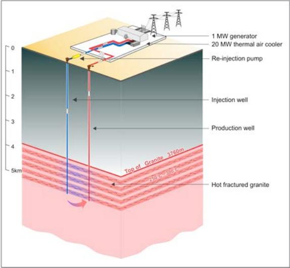
Figure 4-21: Diagram of an Enhanced Geothermal Power Plant (Source: Science.org Australia)
