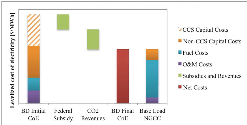
Fig. 3. Relative levelized cost of electricity estimates of the Boundary Dam retrofit by cost category compared to a base load NGCC plant [14]
