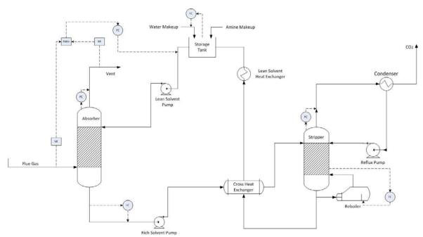
Figure 2. Absorber/stripper process flow diagram with control structure
