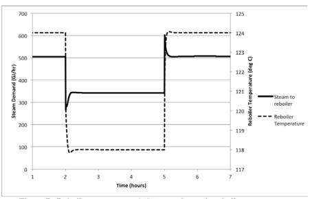
Figure 7. Reboiler response to -/+5% step change in reboiler temperature
