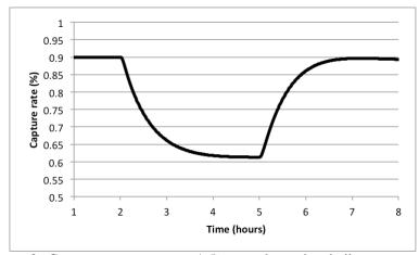
Figure 8. Capture rate response to -/+5% step change in reboiler temperature
