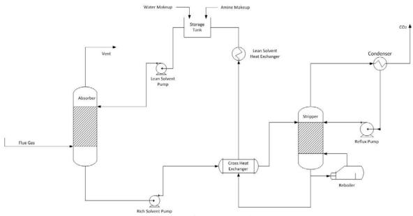
Figure 1. Process flowsheet for absorber/stripper post-combustion capture process
