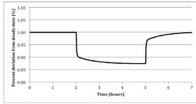
Figure 5. Change in lean solvent flow for flue gas disturbances.
