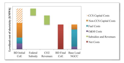
Fig. 3. Relative levelized cost of electricity estimates of the Boundary Dam retrofit by cost category compared to a base load NGCC plant [14]
