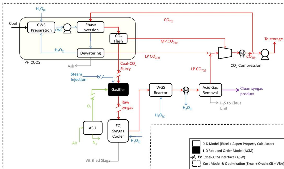
Figure 4: Scope of syngas production plant considered and summary of tools used for the analysis. Coal preparation and handling, ash handling, and Claus unit were not modeled but are included in the cost model.
