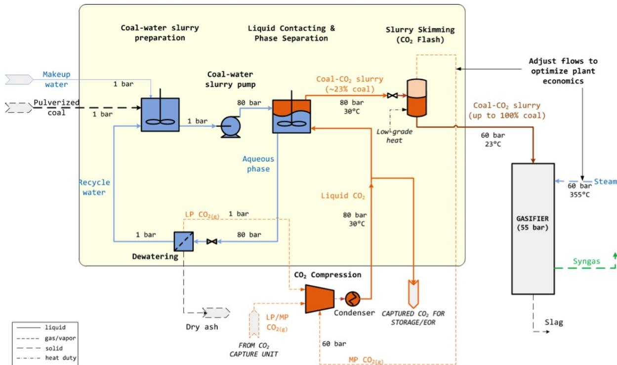
Figure 3: PHICCOS-fed gasifier with CO<sub>2</sub> slurry skimming and steam injection.
