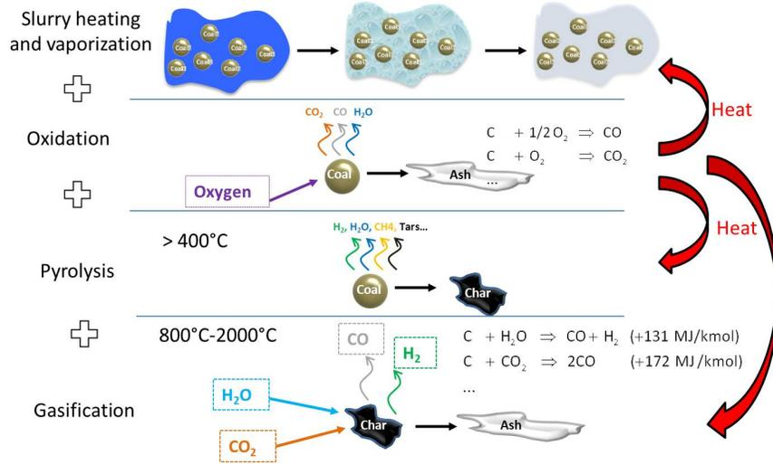
Figure 1: Schematic of autothermal operation of an oxygen-blown, entrained flow coal gasifier.
